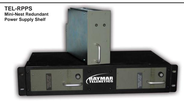
The Mini-Nest Redundant Power Supply Shelf was designed to provide redundant power to existing Mini-Nest installations. The shelf has both horizontal or vertical mounting options to fit into existing data cabinets. The inter-connect cable is available in a variety of lengths allowing the shelf to be installed some distance from the exiting nest.
